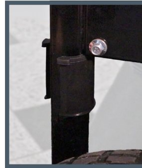
Fig. B - Rubber Sleeve around square tube with mouth facing out
