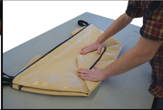
5. Fold canopy so that top cap is in the center of canopy. Ensure the top cap ends are flat & not flipped upward.
